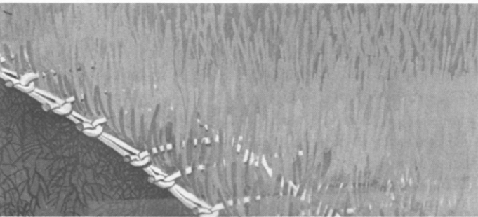
Fig. 5. Use of mulching blanket for dike erosion control (illustration, Gulf States Paper Corporation).
